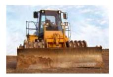
A self-propelled compactor is a tamping foot drum, wheeled machine that is used to compact a variety of civil construction materials.
