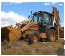
The backhoe/loader loads and pushes materials. The backhoe/loader attachment digs into the ground to excavate materials.
