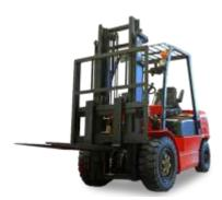
A forklift is a powered industrial truck equipped with a mast and an elevating load carriage with a pair of fork arms or another load handling attachment.
