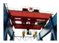
**Bridge Crane** – A bridge beam, mounted at each end to an end carriage, capable of travelling along elevated runways and having one or more hoisting mechanisms arranged to traverse across the bridge.
