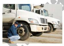
Check that all wheels are secure, wheel rims are not bent or cracked and that there is the correct number and type of nuts and studs.
